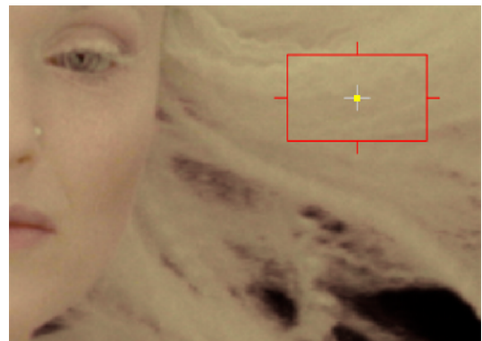
Selecting the hair color despills the blue pixels, producing a better matte.
