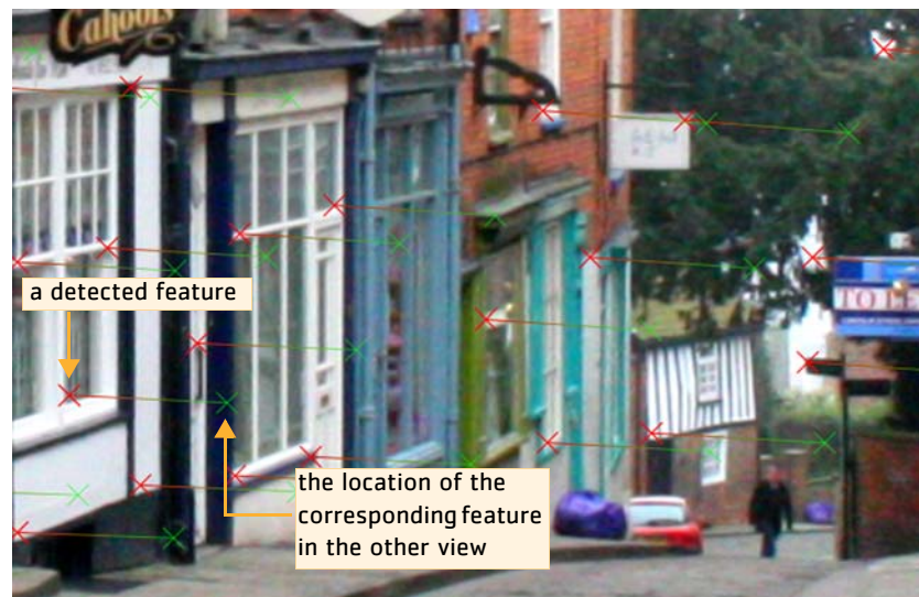
Figure 1. O_Solver detects features in each view and tries to match them.
