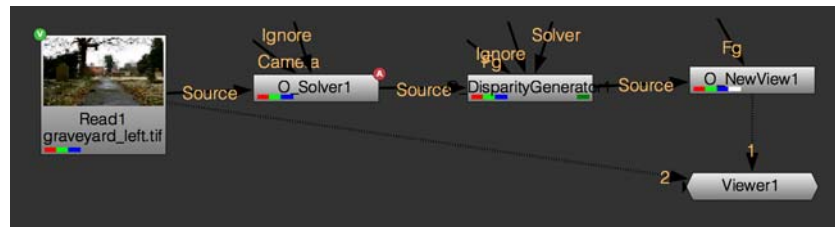
Figure 43. The Viewer here has two inputs: 1) the O_NewView node with the newly generated left view and 2) the Read node with the original left view.
