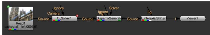
Figure 131. A node tree with O_InteraxialShifter . O_Solver and O_DisparityGenerator are not needed in this tree if the necessary disparity channels are included in the Read node.
