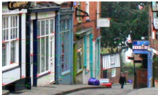
Figure 17. Showing the features and matches for the camera relationship calculation in a Viewer overlay.
