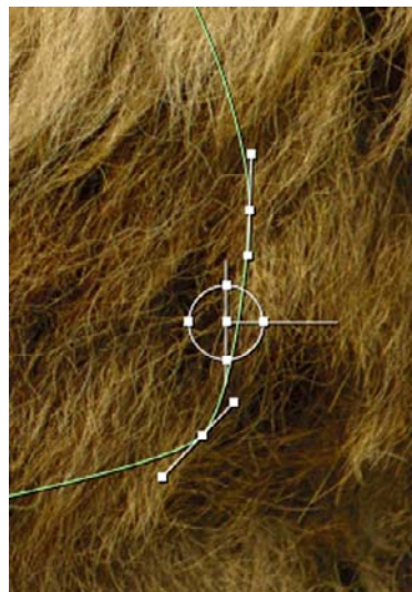
Figure 12.1: To close an open curve or open a closed curve, right-click on a point and select open/close curve .
