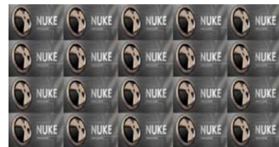
The output of the Tile node with rows set to 4 and columns to 5.
