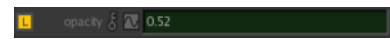
Figure 15.8: A dark green parameter signifies the value for the current frame is interpolated.
