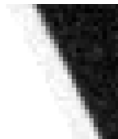
Figure 34. Screen Clip Rollback has been used to reduce the unwanted erosion of the edge.
