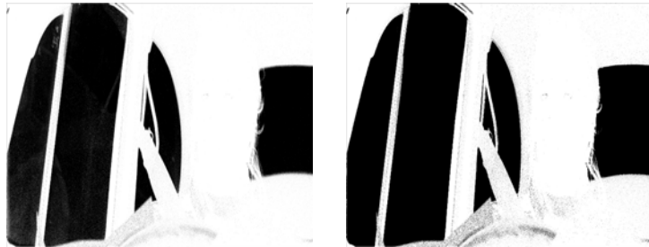
Figure 29. Screen Gain = 105 giving a good screen matte. Figure 30. Screen Gain = 150 giving background show through and over eroded edges.
