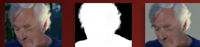
Original image Extracted matte using ColourMatte Output composited over grey
