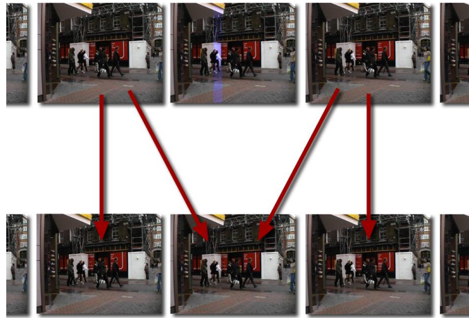
Figure 17.1 Damaged frame (top centre) repaired by taking the previous and next frames to construct the missing frame.
