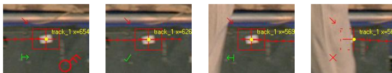
Figure 38.3 (left to right) Start range icon, in range icon (tick), end range icon and out of range icon (cross).
