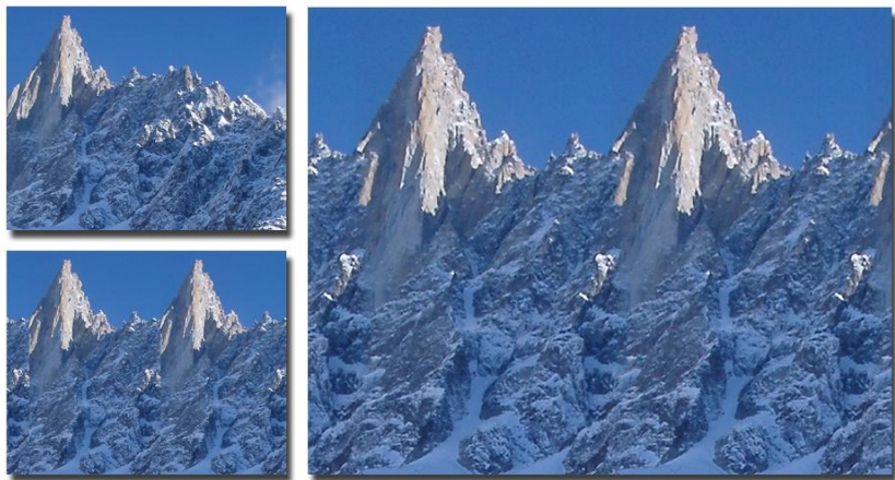
Figure 37.7 Top left is the original image, bottom left a tile with an overlap of zero giving a straight edge. The picture on the right has an overlap of 28 giving a seamless join.
