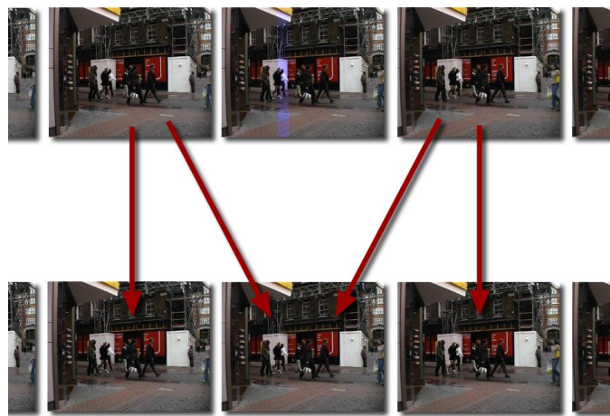
Figure 22.1 Damaged frame (top centre) repaired by taking the previous and next frames to construct the missing frame.
